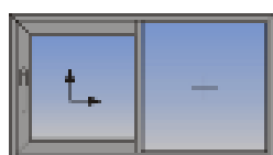
Single L&S sash with fixed
